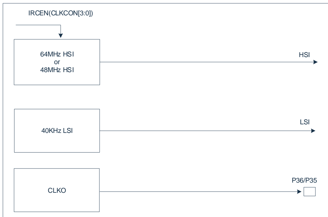
Figure 3-1: Block diagram of the clock structure
